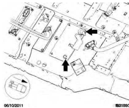
Fig 162, Drain Tube Inspection (from July 2011)
